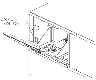
FIG. 44 ON/OFF Switch
